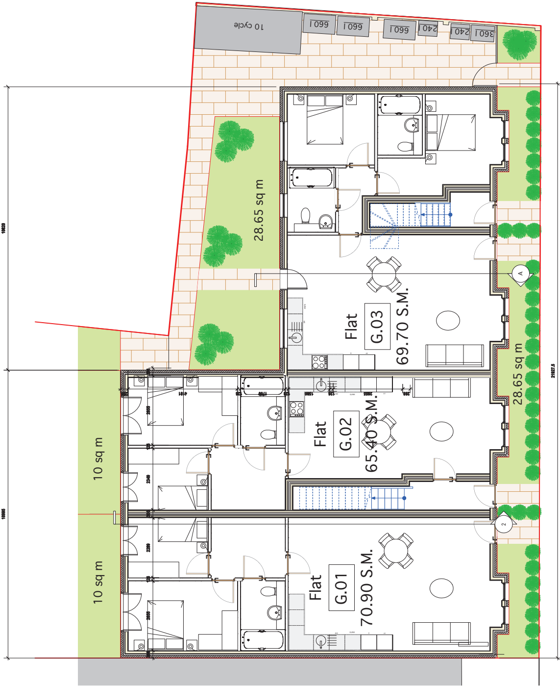
Proposed Ground Floor Plan Scale: 1:50
